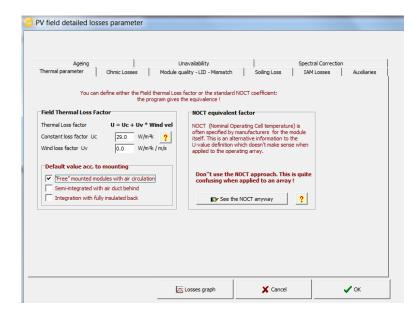
coefficients for use in PVSyst, based on thermal performance of a subset of the SunPower fleet in which the thermal loss coefficients are aligned with PVsyst.
